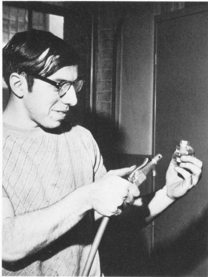
Left:—James Pape, Pipe Shop, demonstrates use of a new special blowgun nozzle that absorbs noise while maintaining performance levels when the compressed air gun is used. It is made at our Fluid Power Division in Wake Forest, North Carolina.
